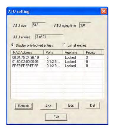
The Address Translation Unit (ATU) performs MAC address searching, learning, and aging functions for all ports of the NJ220 IntelliJack. By default, the ATU table allows a total of 512 entries and an aging time is 304 seconds for each entry.
